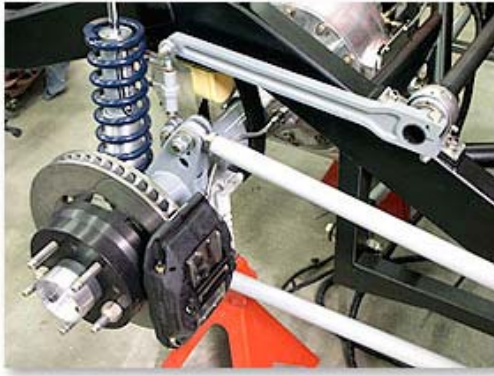
Rear suspension uses a 4-bar setup which can be adjusted for traction. Rear half of frame is custom built. Quick-change rear is suspended by Progress Group coilovers.
