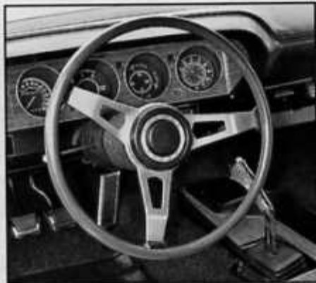
Four-speed Challenger came with cloth seats. Rally dash features separate clock, tach, and four gauges. Wheel's rim-blow.
